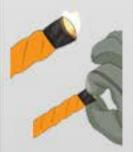
STEP #4: Blow out the flame at the end of the rope that was just cauterized. While wearing a durable leather safety glove, like the ones sold on www.PlankSupply.com, tap the burnt end of the rope to push all of the melted fiber together. Let the rope cool before use. Once cooled, remove the electrical tape.
