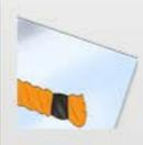
STEP #3: Set the taped piece of rope on a piece of glass. The hot knife will not singe glass like it would other surfaces, such as rubber, plastic, or wood.
