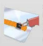
STEP #4: Once the knife tool has heated up, press the heated blade to the middle of the taped off section of synthetic rope. The synthetic rope should begin to melt and seperate. Cut the synthetic rope into 2 seperate pieces. Place the unplugged hot knife tool down on the glass surface to cool.
